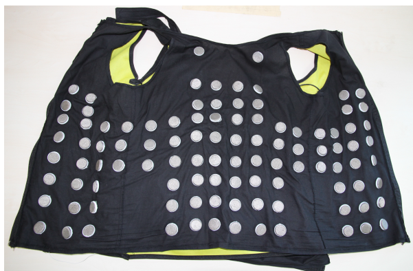
Figure 1: Developed vest with 102 textile electrodes.
