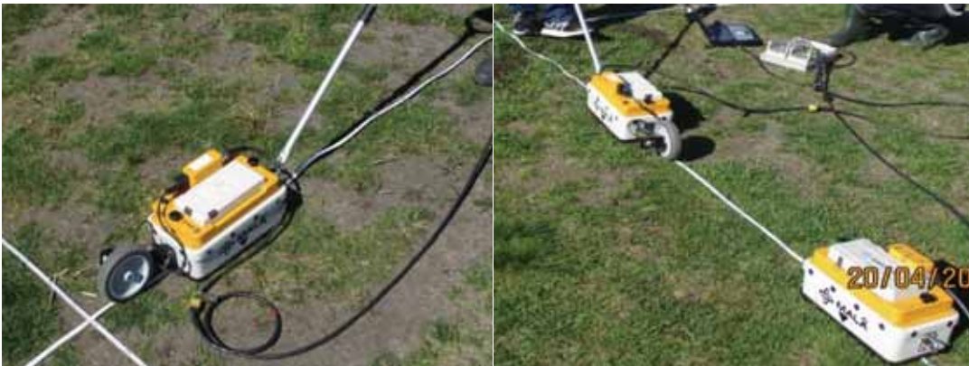
Fig. 2. GPR field data acquisition techniques: a) constant offset reflection b) WARR
