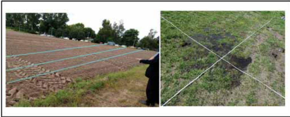
Fig. 1. GPR field measurement layout: a) Measurement traverses across the compacted soil with tractor tires at different passes; b) soil matric potential test point software developed by Sandmeier incorporation
